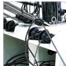
Carbon fibre cam C-Cleat™
