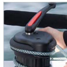
Secure, auto-insert locking mechanism
